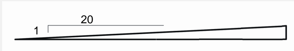
Sloped Pathway – 1 in 20 No distance limit
