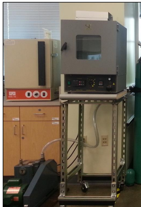
Figure 6: Vacuum Oven for electrode drying.
