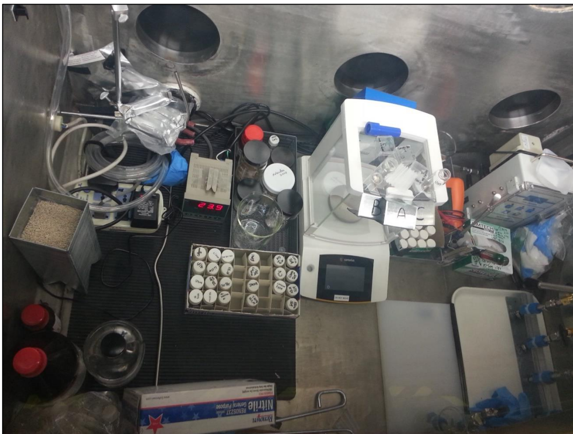
Figure 13: Working chamber layout featuring the internal scale, the cutting pad, the desiccant filter and the O 2 /H 2 O sensors.
