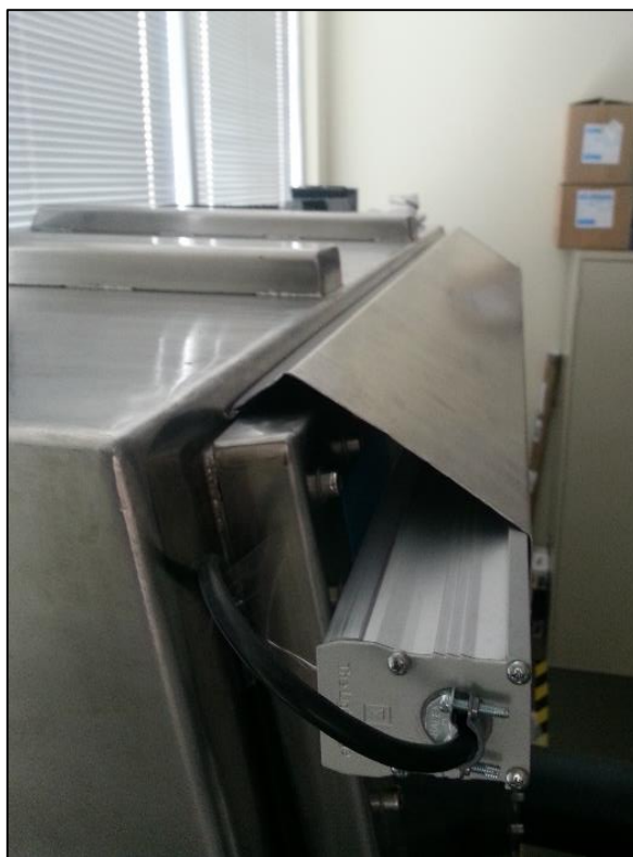
Figure 14: Light fixture for the glovebox.
