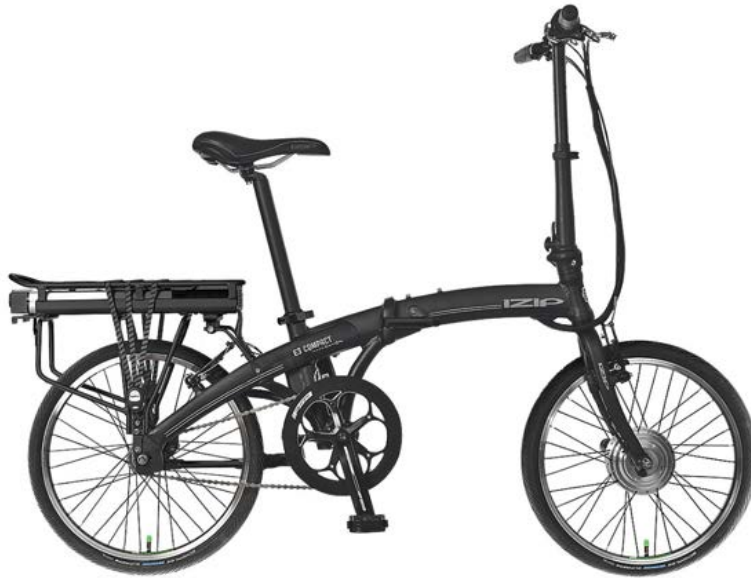
Figure 3-1: Currie iZip E3—a hybrid PB/PAB folding electric bicycle. Image source: CurrieTech.com
