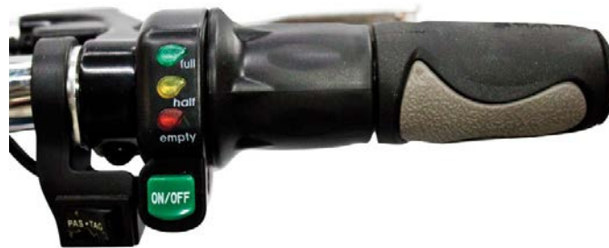
Figure 2-1: A common throttle mechanism for powered bicycles. Image source: CurrieTech.com
