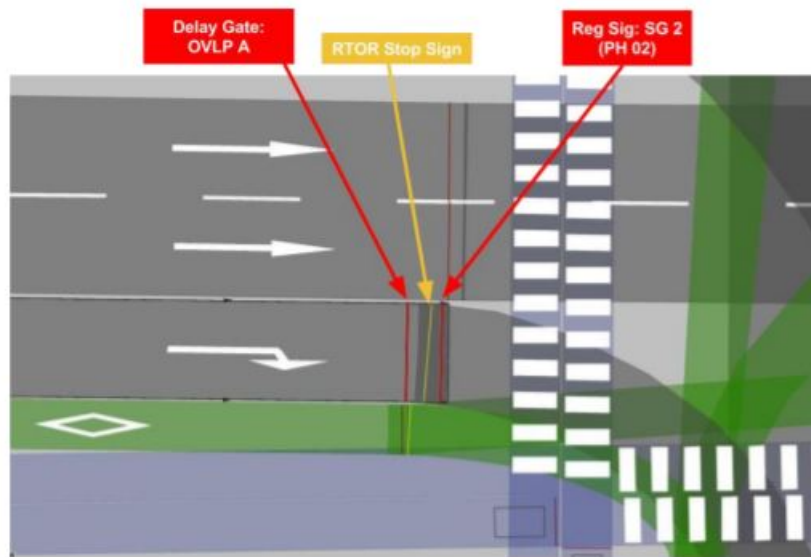
Figure 3.6: Delay Gate Setup in VISSIM
