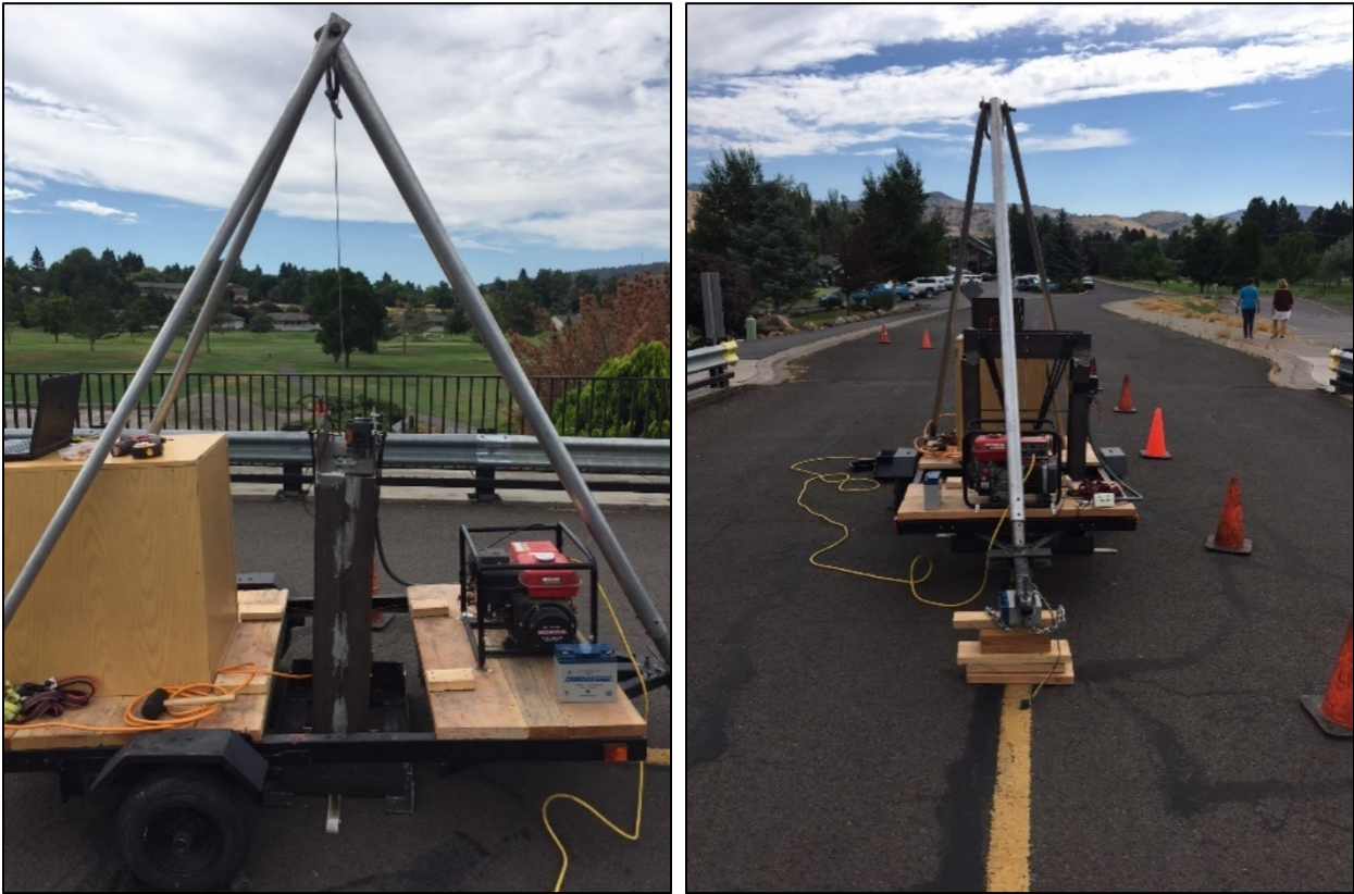
Figure 2.3: Elevation views of tripod-supported heavy shaker frame in RDSETGO Iteration 2.
