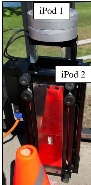
Figure 4.4: iPod placement for shaker/iPod calibration.
