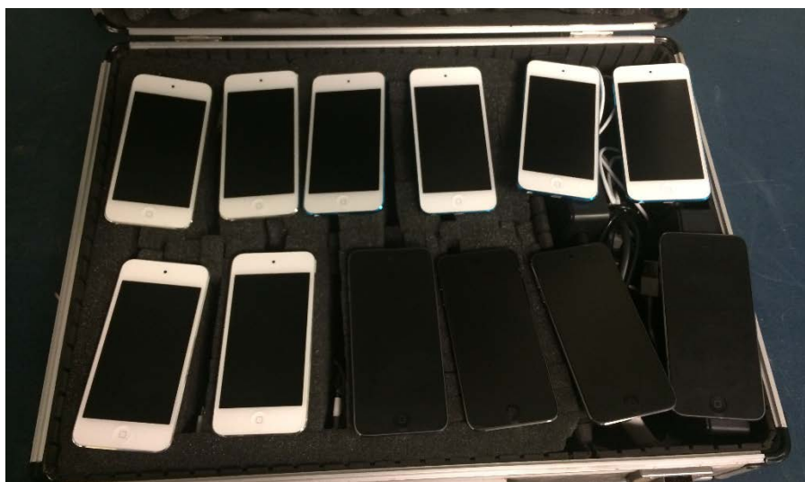
Figure 1.2: 3 rd Generation iPods for acceleration data collection
