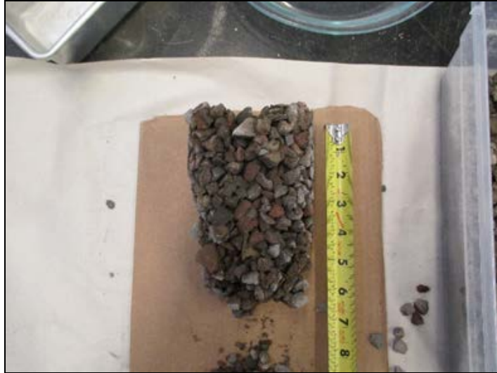
Figure 16 – Bound portion measurement for slurry mix sample SC200.2
