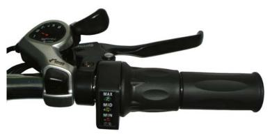
Figure 1: A common throttle mechanism for powered bicycles. *Image source*: E-Republic.co.uk
