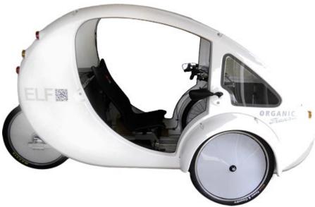
**Figure 5**: Organic Transit's ELF, which is a *low-speed electric bicycle* as defined by CPSC, despite its bulk. *Image source*: OrganicTransit.com
