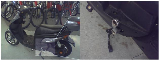
**Figure 20:** Photograph of McClain's scooter-style electric bicycle with a broken pedal. The imprint reads *XL500W*, which corresponds to an EW-600 model of manufacturer Electric Wheels. *Image source*: Officer Michael Massey, Springfield Police, edited by authors.
