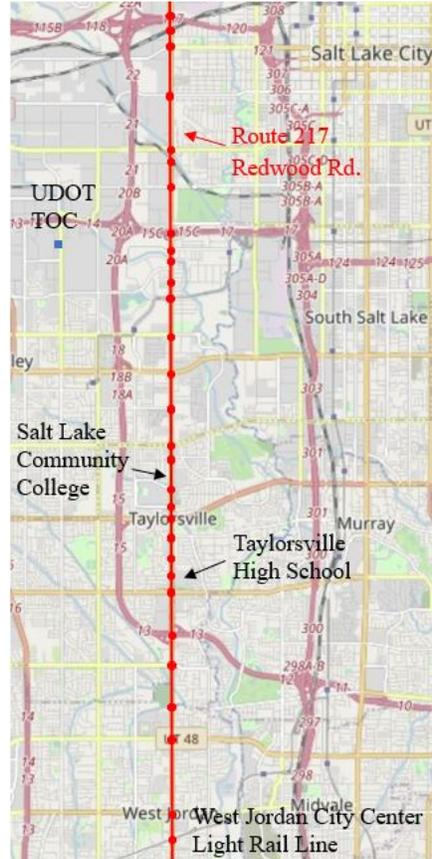
Figure 3.1: DSRC corridor for transit signal priority in Salt Lake City
