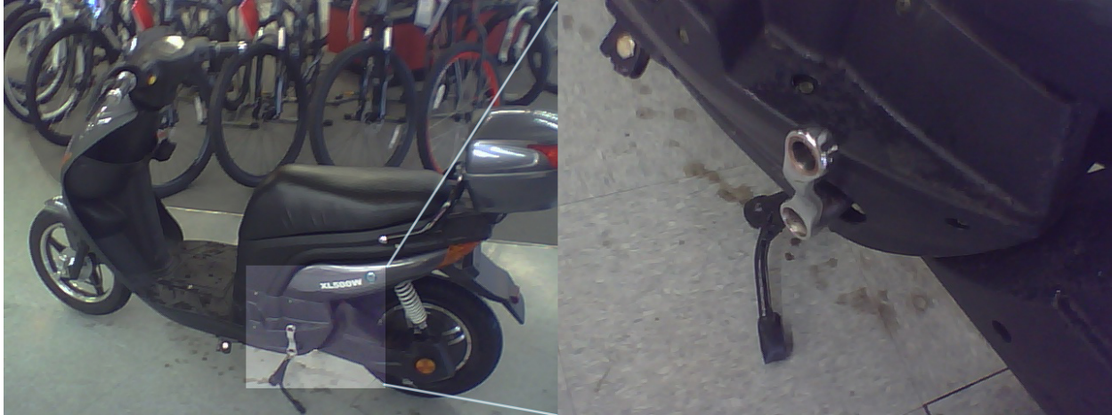
Figure 20: Photograph of McClain's scooter-style electric bicycle with a broken pedal. The imprint reads XL500W , which corresponds to an EW-600 model of manufacturer Electric Wheels. Image source: Officer Michael Massey, Springfield Police, edited by authors.
