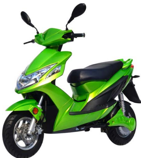
Figure 7: Electric scooter has no pedals, which is not considered an “e-bike.” Image source: Made-in-China.com
