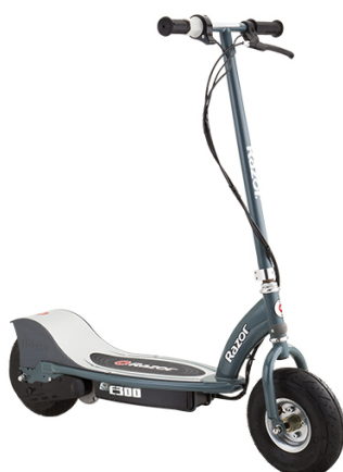
Figure 8: Razor E300 stand-up electric kick-style scooter. This style of kick scooter is not a scooter-style electric bicycle (SSEB). Image source: Razor.com
