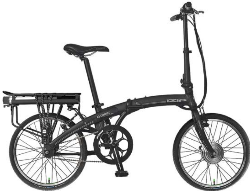
Figure 3: Currie iZip E3—a hybrid PB/PAB folding electric bicycle. Image source: CurrieTech.com
