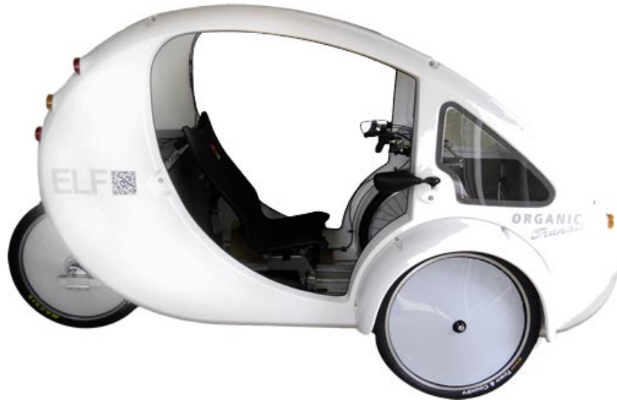
Figure 5: Organic Transit’s ELF, which is a low-speed electric bicycle as defined by CPSC, despite its bulk. Image source: OrganicTransit.com
