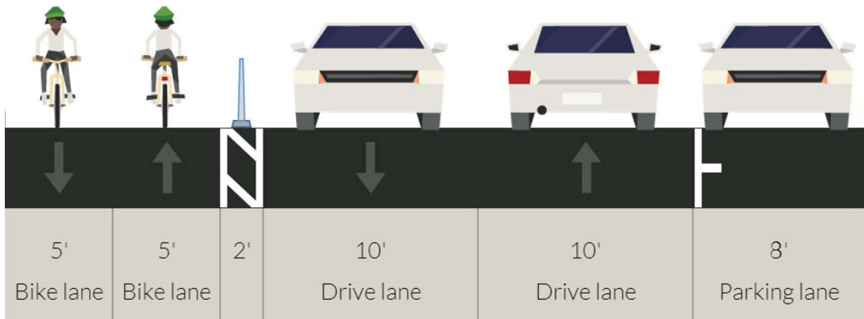
Figure 3-9. Sample Cross section of Bluebonnet Protected Bike Lanes
