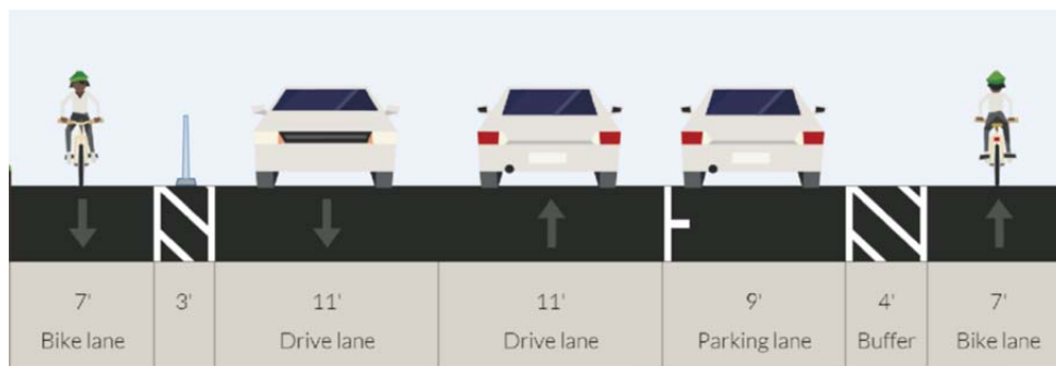
Figure 3-21. Milwaukee Ave. Chicago, IL, Before and After Installation of Protected Bike Lane
