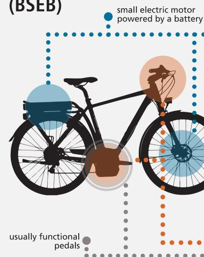
Bicycle-style electric bikes (BSEB) can reach 20 miles per hour when propelled solely by the motor and have a motor of 750 W or less. These bikes have pedals that are meant to propel the bike with or without the help of the motor, which is engaged either automatically (torque or cadence sensor) or with the use of a throttle. BSEBs are distinguished by their ability to be considered bicycles.
