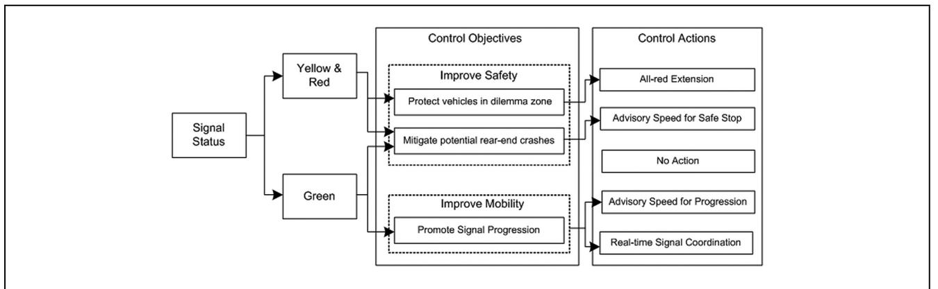
Figure 4. System control actions based on traffic signal status.
