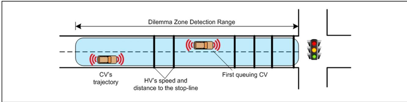
**Figure 3.** Vehicle trajectory information within the detection zone.
