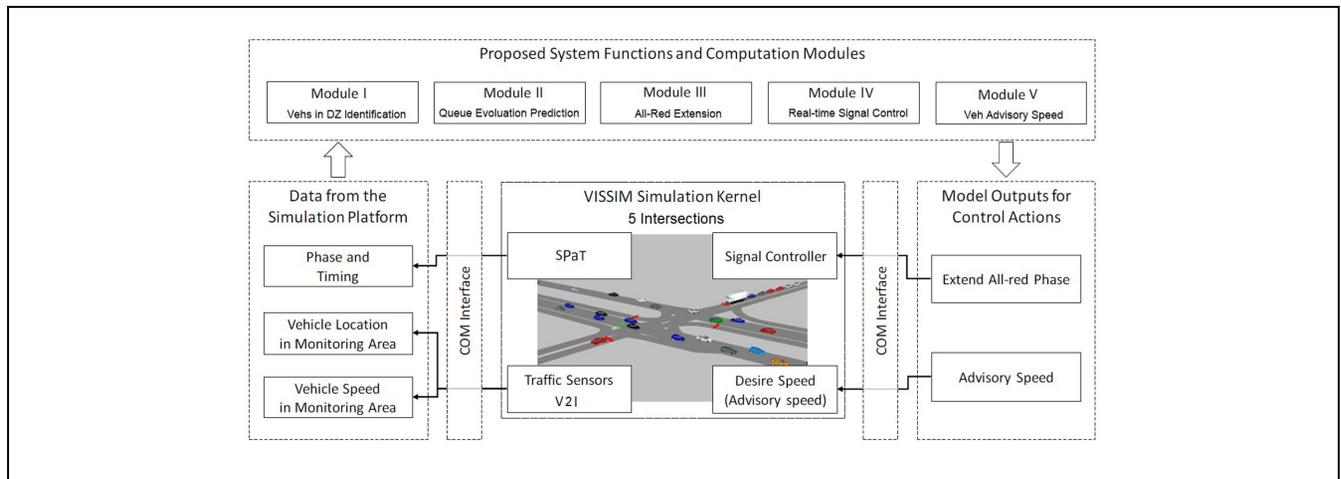
**Figure 6.** Overview of the VISSIM simulation platform.
