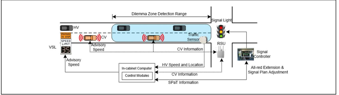
**Figure 1.** Overview of the proposed integrated signal control system.
