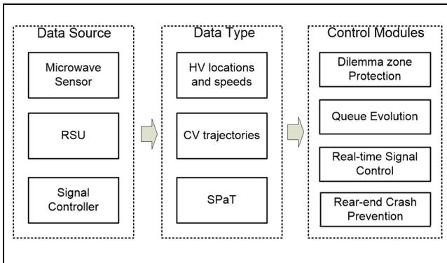
**Figure 2.** Data flowchart of the proposed system.
