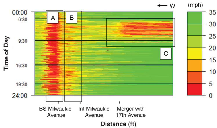
FIGURE 4 Application of numerical method applied to 5 days of bus speeds on a 2,000-ft segment of Southeast Powell Boulevard: (a) bus stop at Milwaukie Avenue, (b) intersection of Southeast Powell Boulevard and Milwaukie Avenue, and (c) merger of 17th Avenue with Southeast Powell Boulevard.
